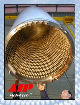
Above: AIP 46" diameter x 80" long Hybrid Inconel-Molybdenum furnace rated for 1225 C. Internal wound for maximum hot zone space.
