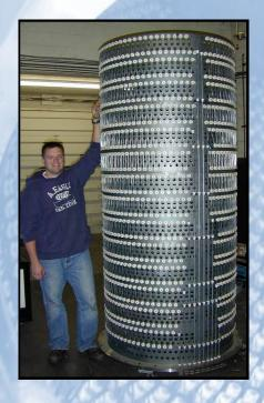
Above: AIP 30" diameter x 80" long Molybdenum furnace rated for 1400 C.
